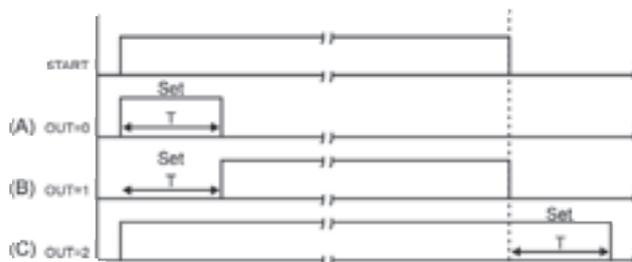
E-75 Series Timer is a single output general purpose timer which can be easily configured by the user. The start signal is generated upon applying 220 V AC to the START inputs. The output forms depending upon the “out” parameter are shown above.
