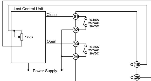
As shown in figure, control of the feedback controlled valve can be made with a servomotor connected to the relays and the 19-20th terminals on E-200, and a potentiometer (1k-5k).
