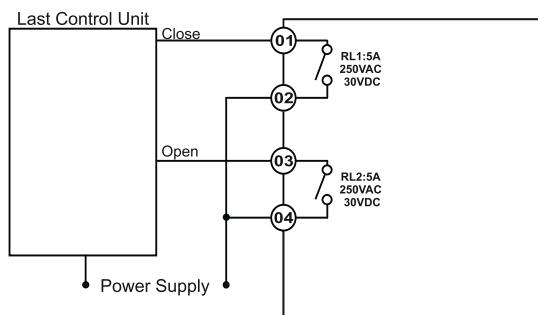
Using the relays on E-200, an open-loop valve control can be made, as shown in figure. Parameters related with this control, are the  $\text{ETYP}$ ,  $\text{dbnd}$  ve  $\text{ErEñ}$  parameters in the  $\text{aLnF}$  page. The explanation for the parameters are;
